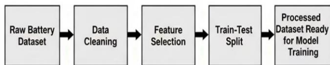
Fig. 2. Overview of the data processing pipeline workflow for lithium-ion battery remaining useful life (RUL) prediction.
